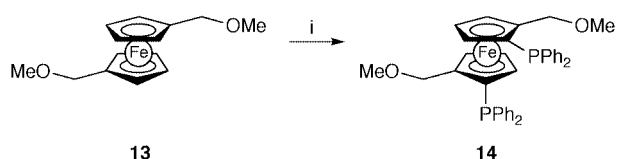
Scheme 7 Reagents and conditions: (i) BuLi, ether, 34 °C, 16 h; Ph 2 PCl, rt, 16 h, 63%.
