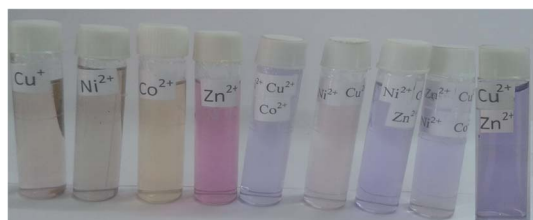
Fig. 14 Color changes observed to H-1 and metal ions ( 1 \times 10^{-4}\text{ M} ) in methanol.
