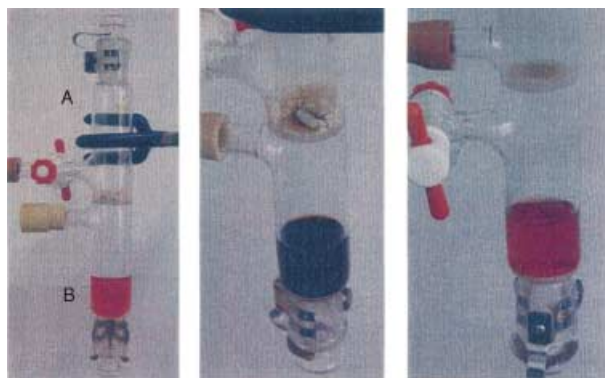
Figure 3. a) Apparatus used for the complexation and decomplexation process, with b) complex 5a in compartment B and c) rotaxane 1a in compartment A after decomplexation.
