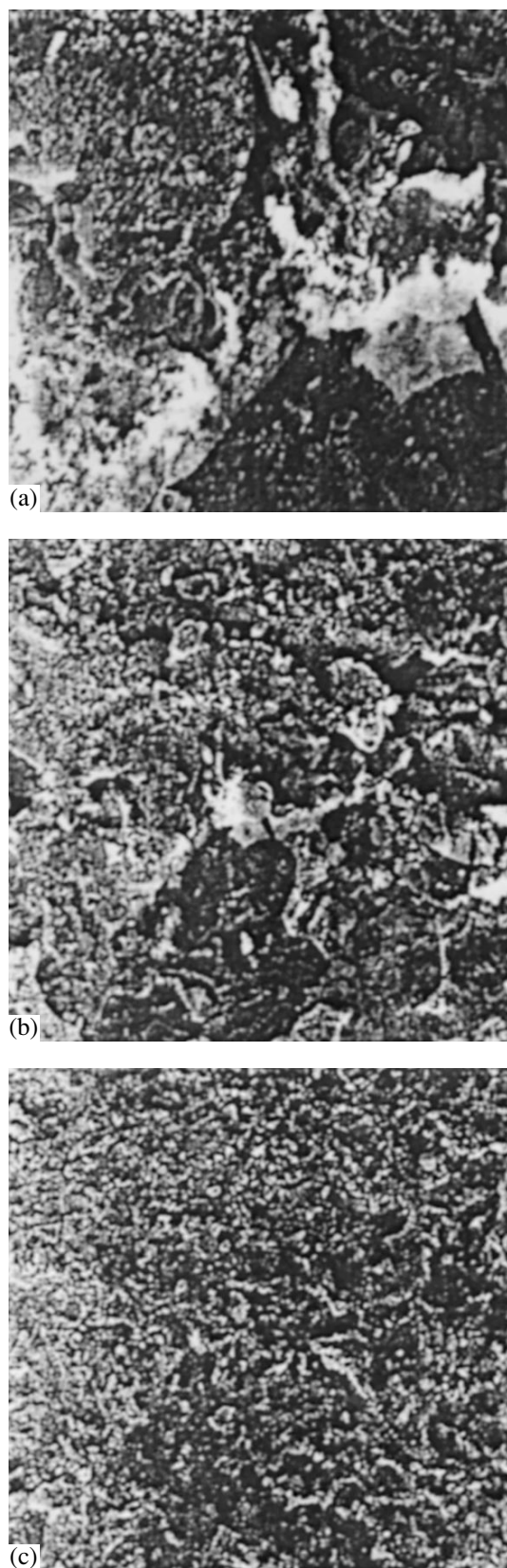
Fig. 4. Micrograph of arsenic deposited on a stainless steel cathode: (a) \times 1000 , (b) \times 300 , (c) \times 100 ; 0.75 M \text{NaH}_2\text{AsO}_3 , j = 0.05 \text{ A/cm}^2 , electrolysis duration of 0.5 h.
