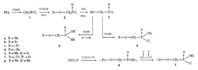
Methyl phosphorodichloridite **1** was obtained in high yield from the reaction of methanol with a 50% excess of phosphorus trichloride ( $\delta$ , 13). The resulting binary mixture of **1** (65 wt %) and phosphorus trichloride was reacted in the next step. This procedure obviated a tedious fractional distillation which unpredictably caught fire owing to the formation of a pyrophoric residue.
