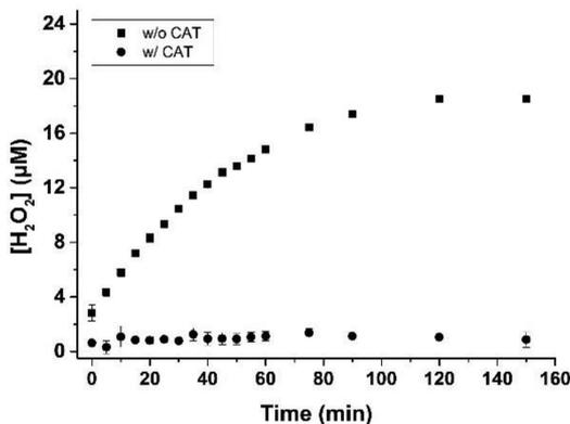
**Figure 4.** Time-dependent generation of  $\text{H}_2\text{O}_2$  from thioglucose ( $100 \mu\text{M}$ ) and GOx ( $10 \mu\text{g}/\text{mL}$ ) in PBS buffer ( $50 \text{mM}$ , pH 7.4) in the presence and absence of CAT ( $50 \mu\text{g}/\text{mL}$ ). The experiments were performed in triplicate, and results are expressed as mean  $\pm$  SD ( $n = 3$ ).
