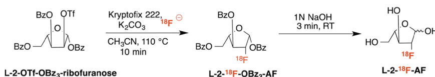
FIGURE 2 Synthesis of 18 F-labeled arabinofuranose-derived structures. A, D-5- 18 F-AF and L-5- 18 F-AF radiosyntheses B, D-2- 18 F-AF and L-2- 18 F-AF radiosyntheses
