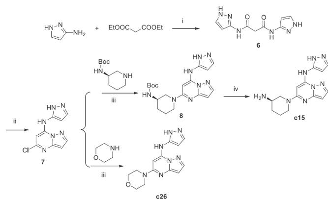
**Scheme 2.** i. 130 °C, neat; ii. POCl<sub>3</sub>, *N,N'*-dimethyl-aniline, 100 °C; iii. *N,N'*-dimethyl-aniline, DMF, 90 °C; iv. TFA, DCM.
