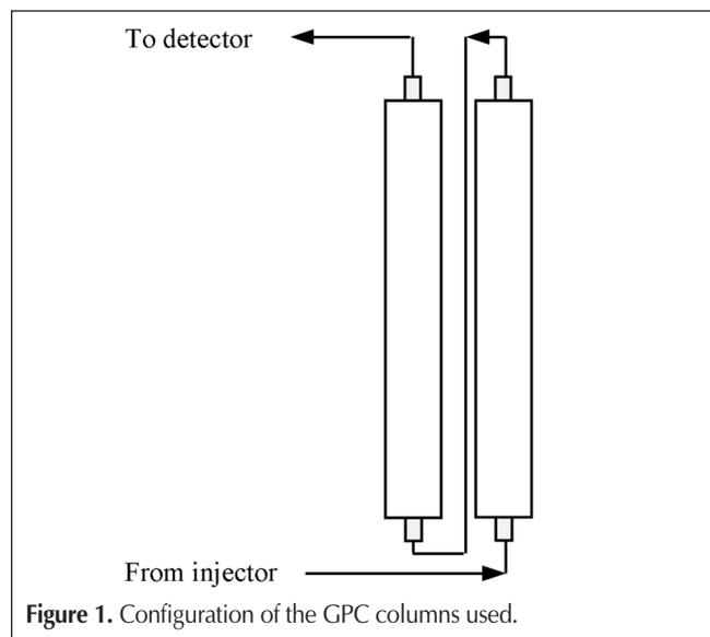
Figure 1. Configuration of the GPC columns used.
