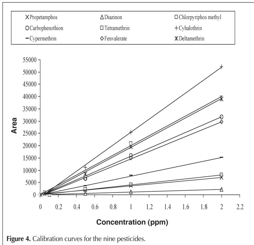
Figure 4. Calibration curves for the nine pesticides.
