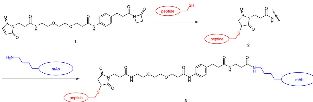
**Scheme 1** Conjugation process between linker **1**, a peptide, and a monoclonal antibody (mAb) to provide bioconjugate drug substance **3**
