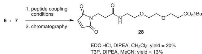
**Scheme 8** Initial amide bond formation conditions for the coupling of acid **6** and amine **7**
