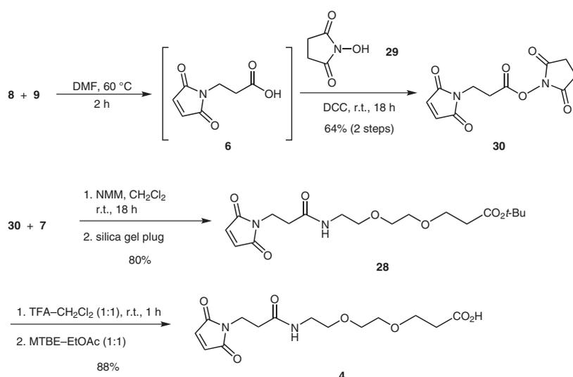
**Scheme 9** Final coupling conditions between acid **6** and amine **7** and *tert*-butyl ester cleavage to give acid **4**
