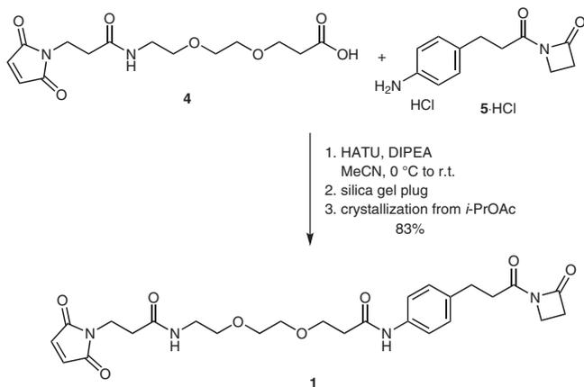
**Scheme 10** Optimized coupling conditions between acid **4** and aniline hydrochloride **5** to produce linker **1**
