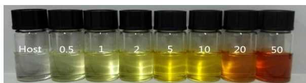
Fig. 3 Naked-eye color changes of SA ( 5 \times 10^{-3} mol/L) with subsequent addition of TNT from 0.5 to 100 equiv under visible.
