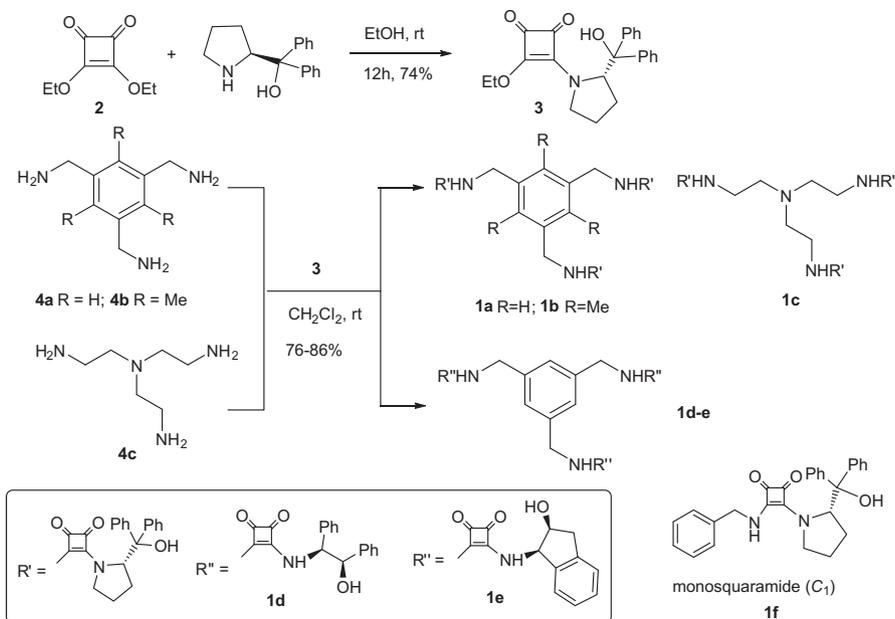
Scheme 1. Preparation of  $C_3$ -symmetric squaramides **1a-f**.
