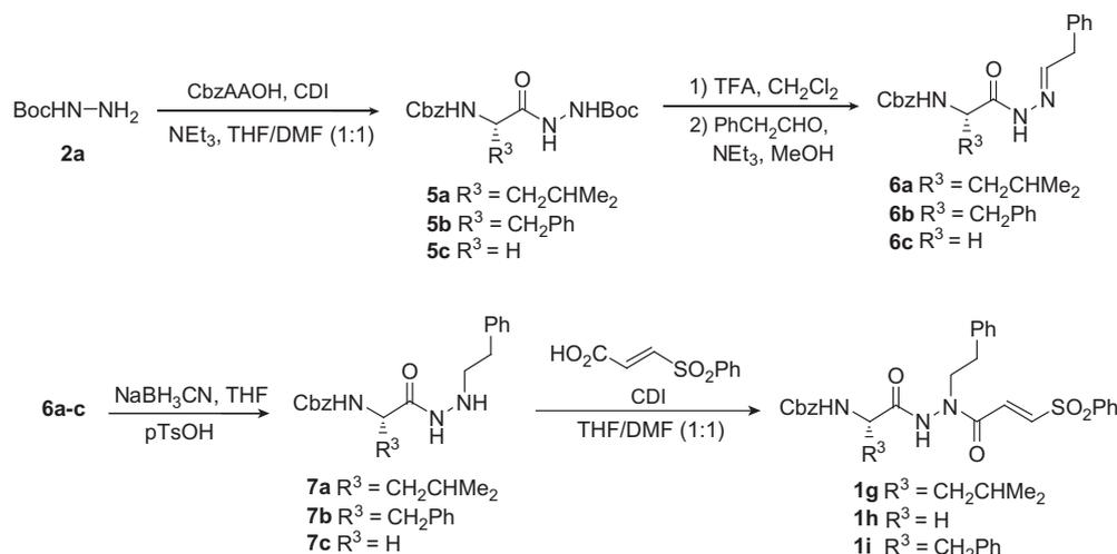
Scheme 3. Synthesis of aza vinyl sulfones **1g–i**.
