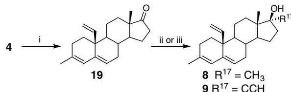
**Scheme 5.** Reagents: (i) TPAP, NMO, 53%; (ii) MeMgBr, 59%; (iii)  $\text{LiC}\equiv\text{CTMS}$  then MeOH, NaOH, 49%.
