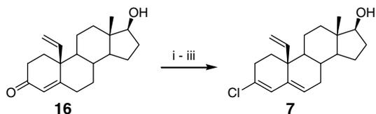
**Scheme 4.** Reagents and condition: (i)  $\text{Ac}_2\text{O}$ , pyridine, DMAP, 100%; (ii)  $\text{POCl}_3$ , AcOH, rt, 50%; (iii) KOH, MeOH, 40%.
