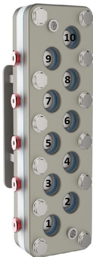
Figure 2: The reaction block from the agitated cell reactor 6 with numbered CSTRs
