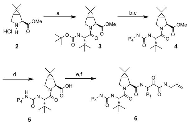
**Scheme 1.** Synthesis of the P3 capped amide and lactam analog of **1**. Reagents and conditions: (a) *tert*-leucine, EDCl, HOOBt, DMF/CH<sub>2</sub>Cl<sub>2</sub>; (b) 4 M HCl/dioxane, rt; (c) P4NCO, DIPEA, CH<sub>2</sub>Cl<sub>2</sub>; (d) LiOH, THF/MeOH/H<sub>2</sub>O; (e) P1 hydroxy allyl amide, EDCl, HOOBt, DMF/CH<sub>2</sub>Cl<sub>2</sub>; (f) Dess–Martin periodinane.
