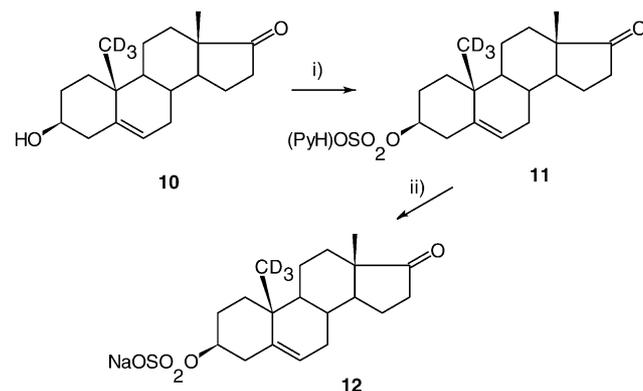
Scheme 5. (i) P<sub>4</sub>ASO<sub>3</sub>, P<sub>4</sub>; (ii) NaCl, H<sub>2</sub>O.
