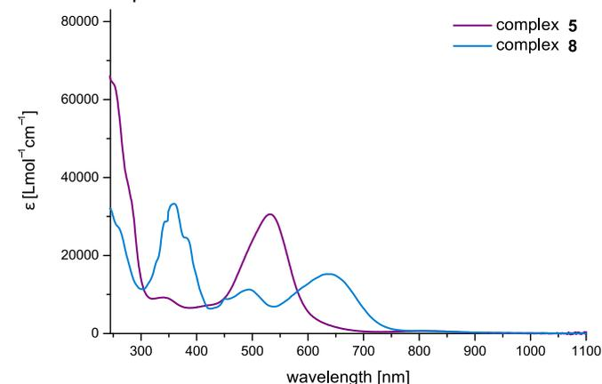
**Fig. 3** UV/Vis absorption spectra of **5** and **8** in  $\text{CH}_2\text{Cl}_2$  (245–1100 nm).
