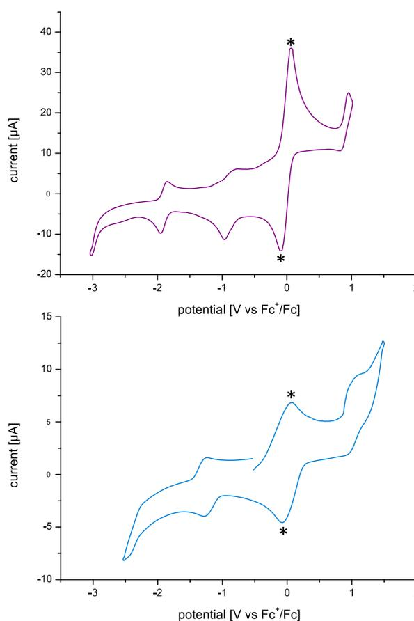
**Fig. 5** Cyclic voltammogram of **5** (top) and **8** (bottom) (0.001 M) on a Au electrode ( $0.1 \text{ V s}^{-1}$ ,  $0.2 \text{ M } n\text{-Bu}_4\text{NPF}_6/\text{CH}_2\text{Cl}_2$ , referenced to internal  $\text{Fc}^+/\text{Fc}$ ). \* marks the redox sweep of the  $\text{Fc}^+/\text{Fc}$  reference redox couple.
