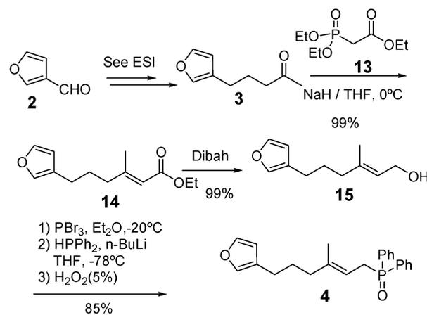
Scheme 2 Synthesis of phosphine oxide **4**.
