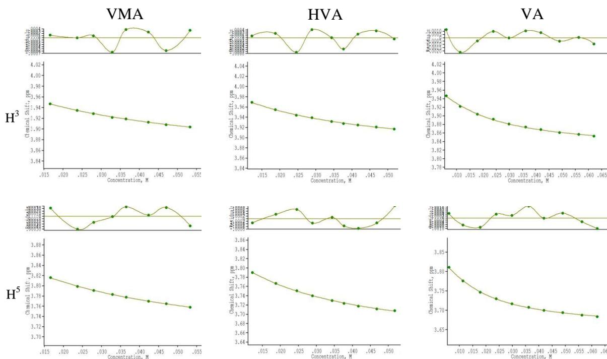
**Figure 2:** Exemplary plots with experimental data and calculated chemical shifts of signals of the  $\text{H}^3$  (upper) and  $\text{H}^5$  (bottom) of the  $\beta\text{-CD}$  together with the residues in magnified form (WinEQNMR program)
