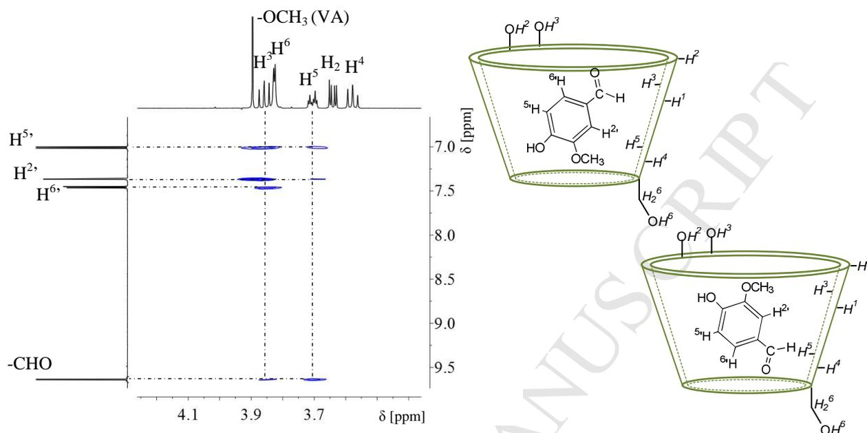
**Figure 5:** Partial contour plot of the two-dimensional ROESY spectrum of 4:1 VA/ $\beta$ -CD ratio and postulated geometry of the complexes
