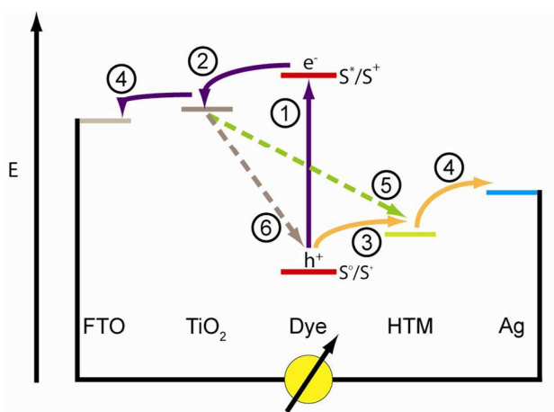
Figure 1. The operating principle of a ssDSSC. 1) Upon absorption of light, the dye generates an exciton; 2) the excited electron is injected into the conduction band of the \text{TiO}_2 ; 3) the dye is regenerated by the hole-transporting material (HTM); 4) the charges percolate to the electrodes. Two common back-reaction processes in ssDSSCs are: 5) recombination of the electrons in the \text{TiO}_2 with the holes in the HTM and 6) reduction of the oxidized dye.
