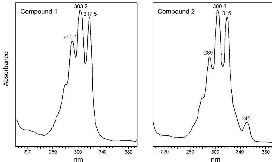
Fig. 3. UV spectra (in methanol) of Compounds 1 and 2 derived from eicosapentaenoic acid.
