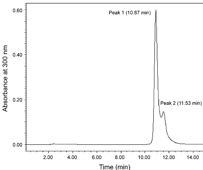
Fig. 2. HPLC analysis of the reaction mixture (following solid phase extraction to remove DBU) of the conjugated fatty acids derived from eicosapentaenoic acid. Column: Nucleosil-C18 (4.6 × 250, 5  $\mu$ m); mobile phase: methanol–water–acetic acid (85:15:0.1); flow rate: 1.5 ml/min; detection: 300 nm.
