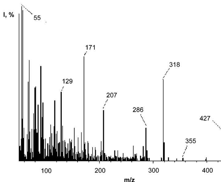
Fig. 4. Mass spectrum of C9–C12 isomer of the MTAD adduct of Compound 2 derived from eicosapentaenoic acid. Molecular  $m/z$  427 and diagnostic  $m/z$  318 ions are clearly visible.
