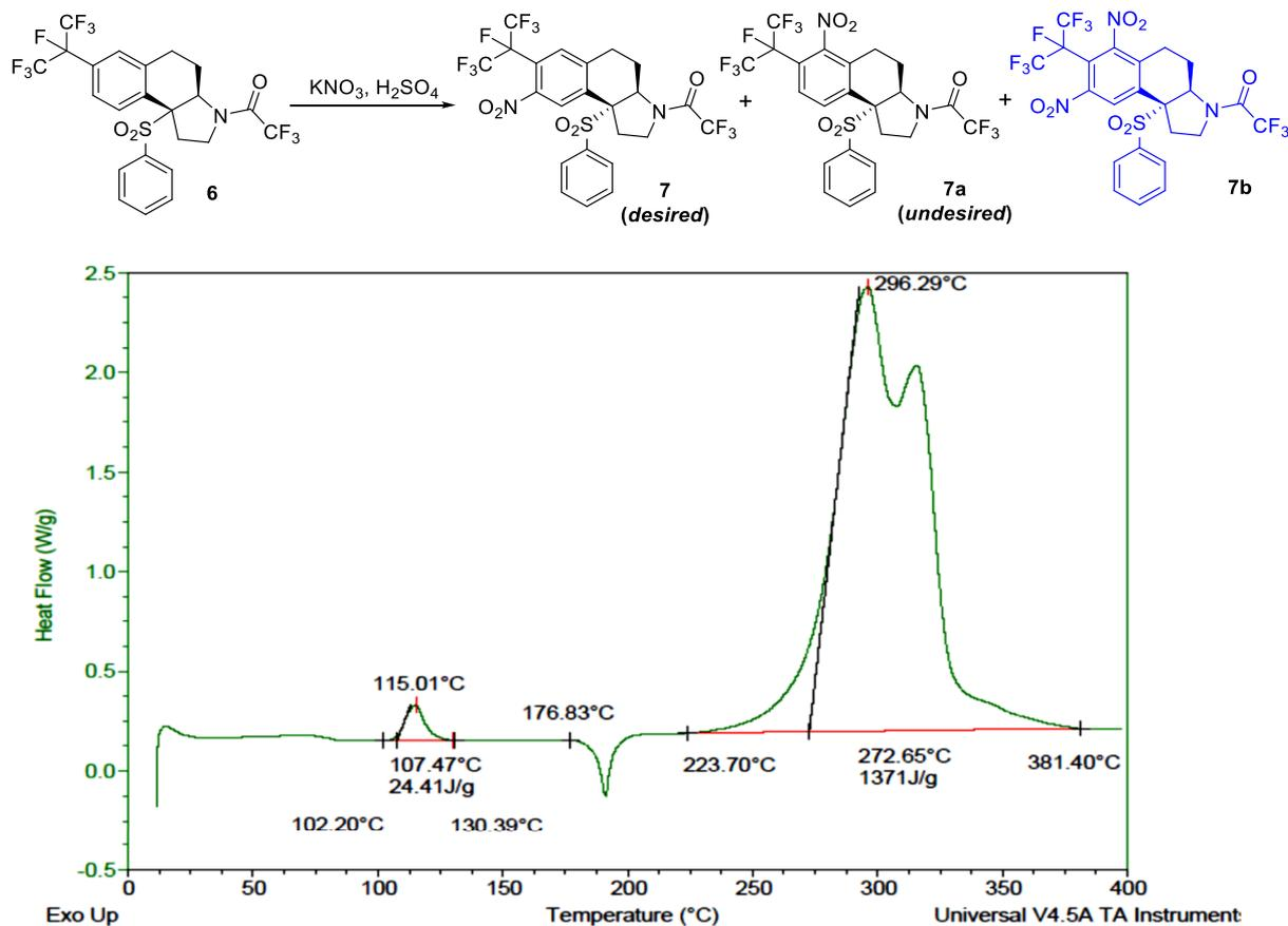
Figure 1. DSC profile of isolated dinitro compound 7b.
