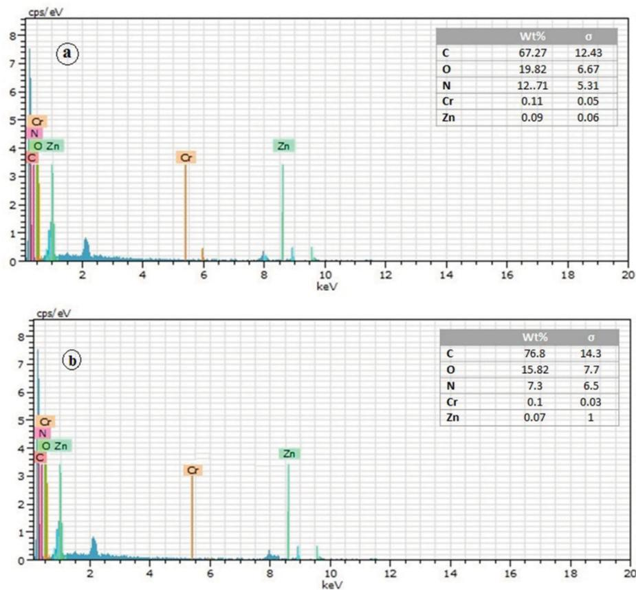
**Figure 4.** EDX spectra of LDHs@PpPDA before (a) and after (b) the reaction.
