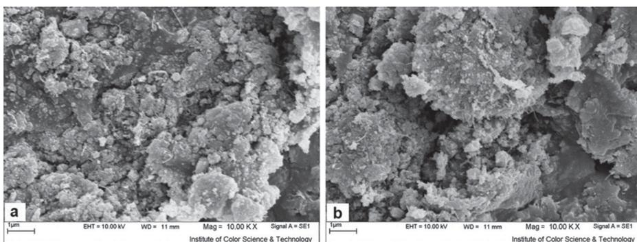
**Figure 5.** SEM images of LDHs@PpPDA before (a) and after (b) the reaction.
