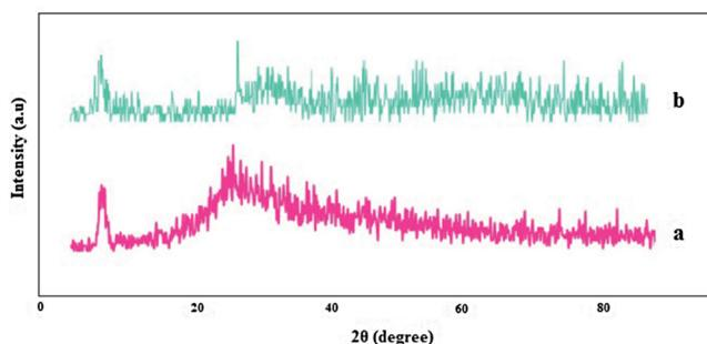
**Figure 6.** XRD pattern of LDHs@PpPDA before (a) and after (b) the reaction.
