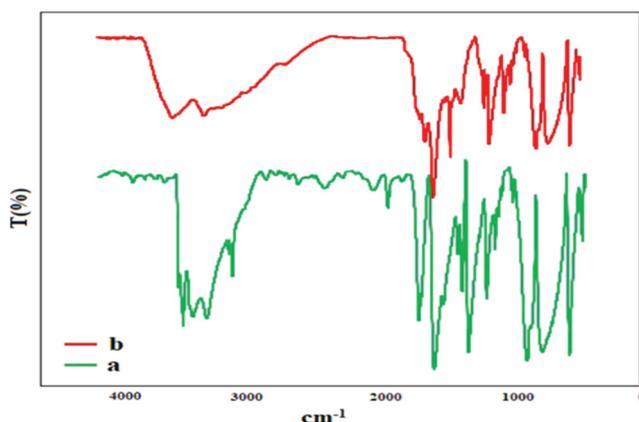
**Figure 3.** FT-IR spectra of LDHs@PpPDA before (a) and after (b) the reaction.
