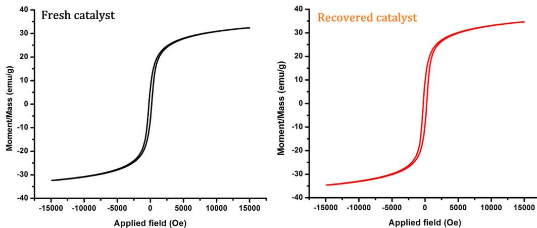
**FIGURE 5** Hysteresis loop of fresh and recovered catalyst
