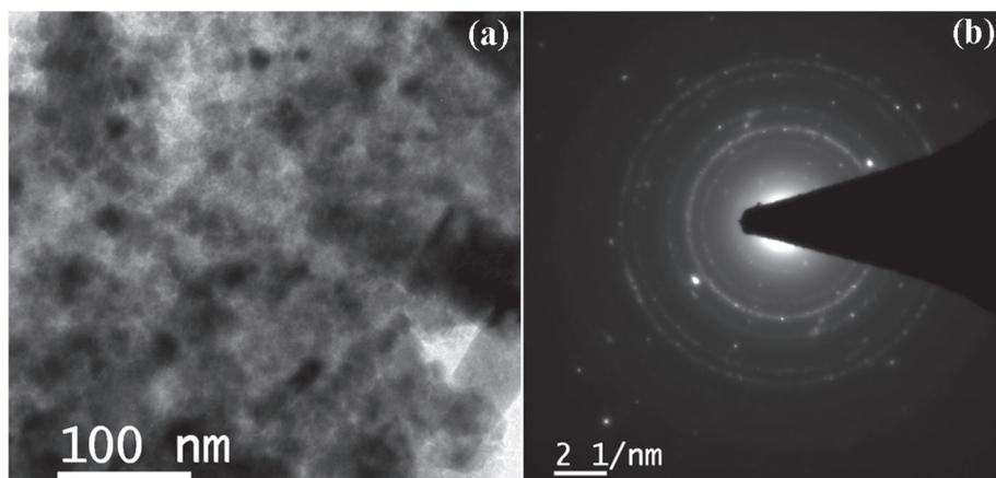
**FIGURE 4** TEM and SAED images of  $\text{CuFe}_2\text{O}_4$  nanoparticles
