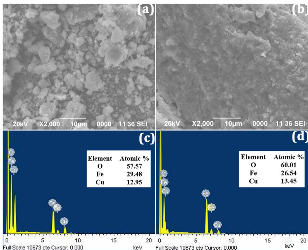
**FIGURE 1** SEM images of fresh and recovered catalysts (a and b); EDX (SEM) spectra of fresh and recovered catalysts (c and d)
