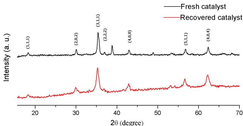
**FIGURE 3** XRD spectra of fresh and recovered catalysts
