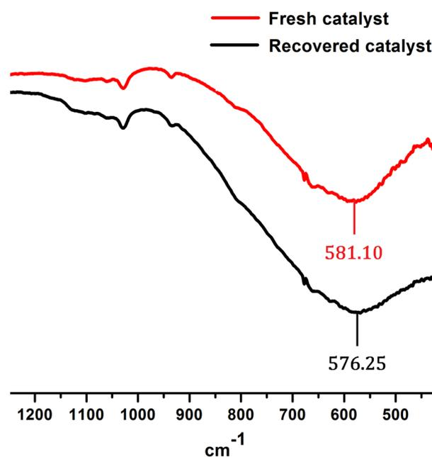
**FIGURE 2** FT-IR spectra of the fresh and recovered catalyst
