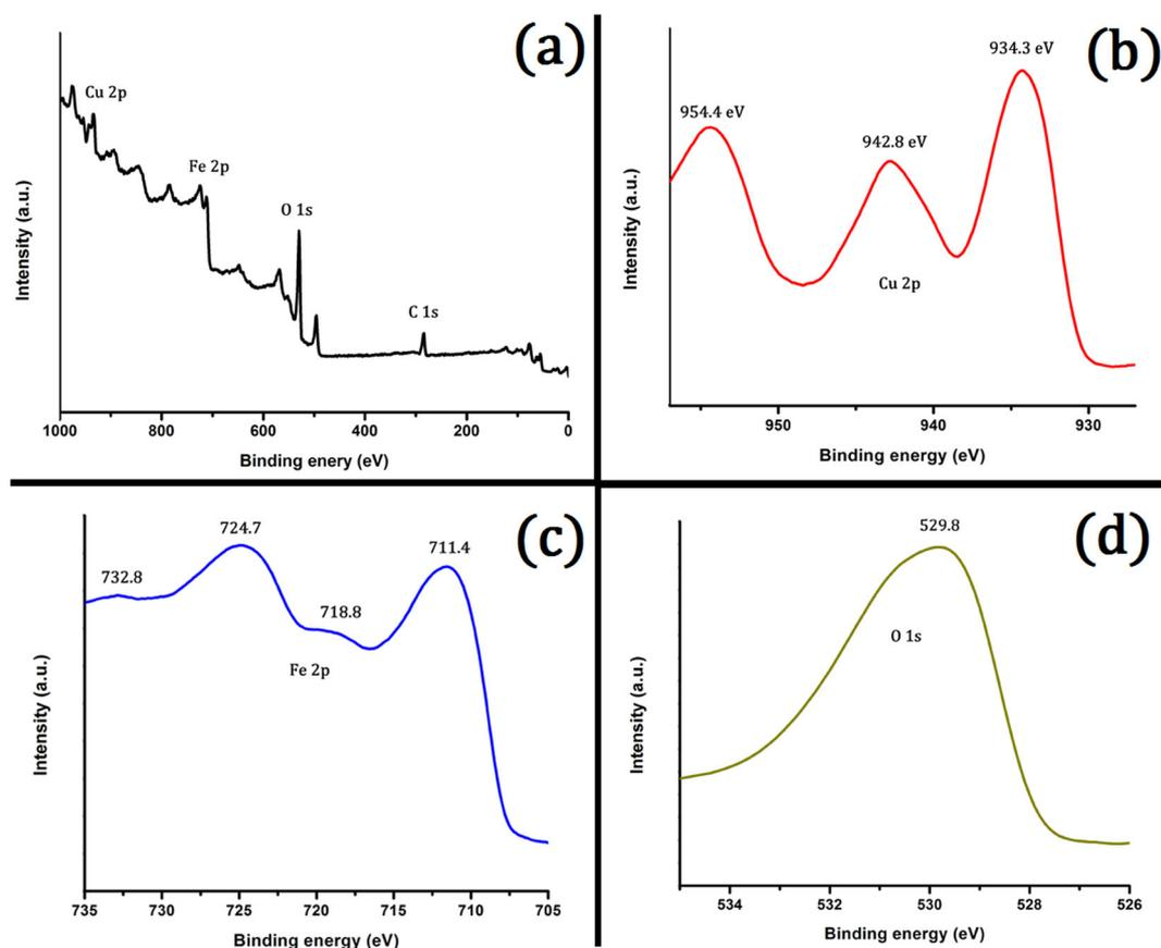
**FIGURE 6** XPS spectrum of prepared  $\text{CuFe}_2\text{O}_4$ : Survey spectrum (a); high resolution spectrum of Cu 2p (b), Fe 2p (c) and O 1s (d)
