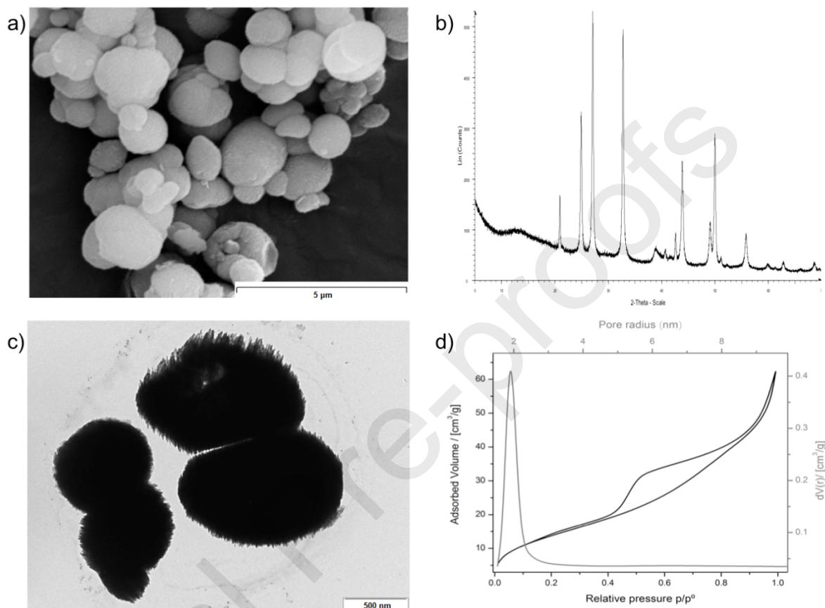
**Figure 2. a) SEM image of Support-a, b) Powder X-ray diffraction (PXRD) of Support-a, c) TEM image of Support-a, d) N<sub>2</sub> adsorption/desorption isotherm of Support-a.**
