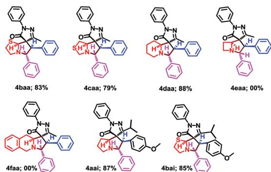
Scheme 4 Substrate scope with different cyclic  $\alpha$ -amino acids. Reaction conditions: **1a** (1.0 mmol), **2a** (1.0 mmol), **3a** (1.0 mmol)  $\text{CHCl}_3$  (3.0 mL),  $75^\circ\text{C}$ , 1 h; under  $\text{N}_2$  atmosphere.
