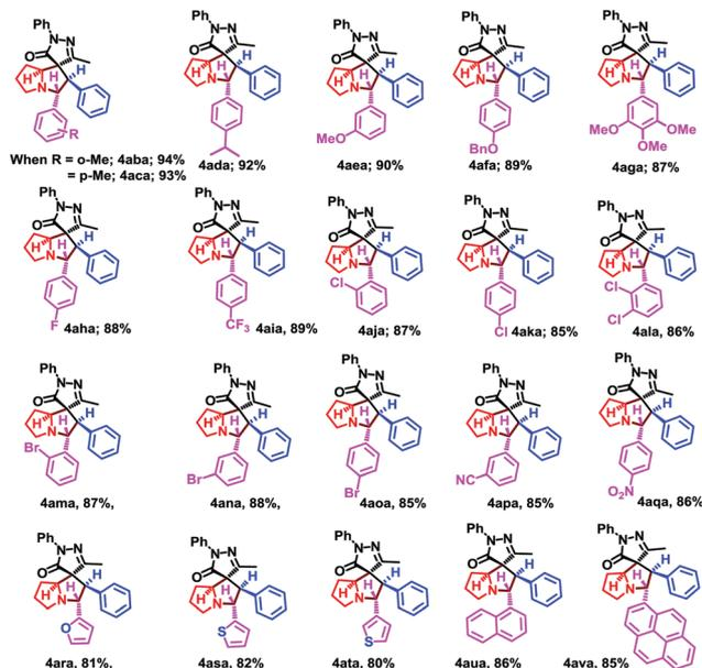
Scheme 2 Substrate scope with respect to various aldehydes. Reaction conditions: **1a** (1.0 mmol), **2a** (1.0 mmol), **3a** (1.0 mmol); anhy.  $\text{CHCl}_3$  (3.0 mL),  $75^\circ\text{C}$ , 1 h, under nitrogen atmosphere.
