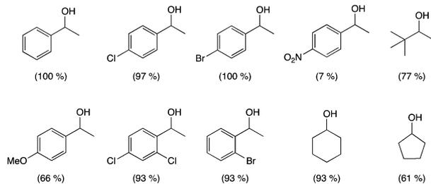
Fig. 8 Formation of alcohols, reagents and conditions: ruthenium complex **4a** (1 mol %), ketone (1.0 mmol), base (0.25 mmol), <sup>i</sup>PrOH (5 mL), 100 °C, 2 h. The conversions were determined by <sup>1</sup>H NMR spectroscopy.
