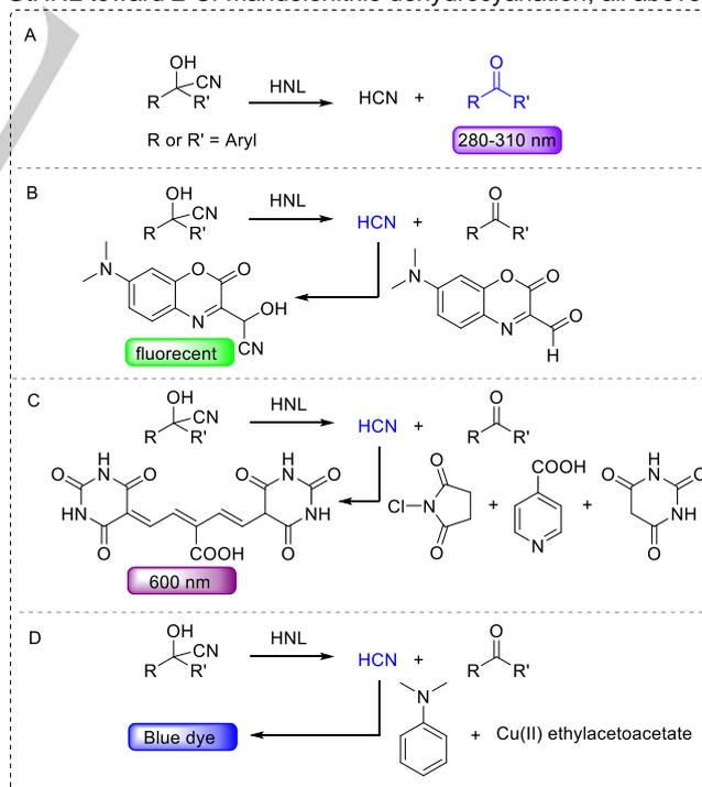
**Scheme 1.** Examples of colorimetric assays reported based on cyanohydrin cleavage. (A) UV absorbance of aromatic aldehydes. (B) Coupling the fluorescent probe. (C) König reaction assays. (D) Feigl–Anger reaction assays.
