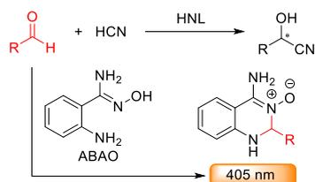
**Scheme 2.** Quantification of residual aldehyde after cyanohydrin synthesis using chromogenic reagent ABAO.
