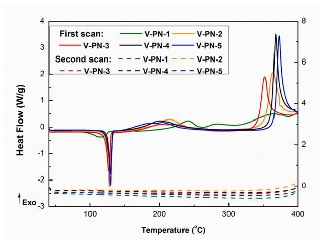
Fig. 2. DSC curves of V-PN resins at a heating rate of  $5\text{ °C min}^{-1}$  under a flow of nitrogen.
