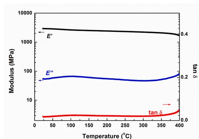
Fig. 5. DMA curves of cured **V-PN-5** resin at a heating rate of 5 °C min<sup>-1</sup> in air.
