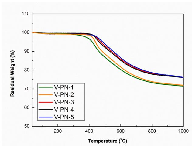
Fig. 4. TGA curves of cured **V-PN** resins at a heating rate of 10 °C min<sup>-1</sup> under a flow of nitrogen.
