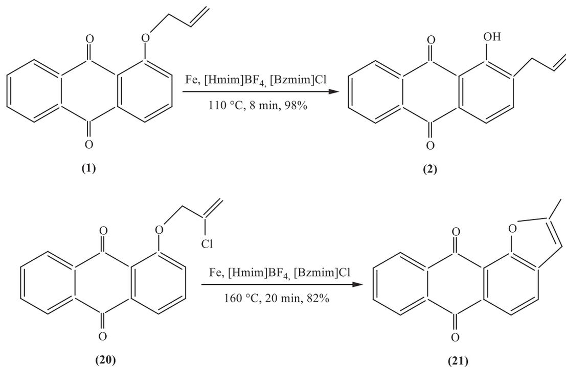
**Figure 1.** Reductive Claisen rearrangement of **1** and **20** to products **2** and **21** respectively using iron powder in a mixture of two ionic liquids, [Hmim]BF<sub>4</sub> and [Bzmim]Cl.
