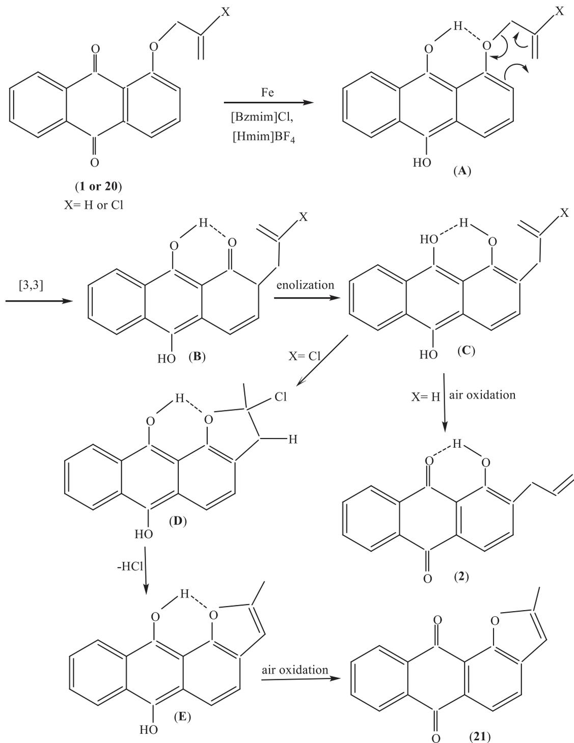
**Figure 4.** The proposed mechanism of the reductive Claisen rearrangement of prop-2'-enyloxyanthraquinones and 2'-chloroprop-2'-enyloxyanthraquinones using Fe/[Hmim]BF<sub>4</sub>/[Bzmim]Cl.
