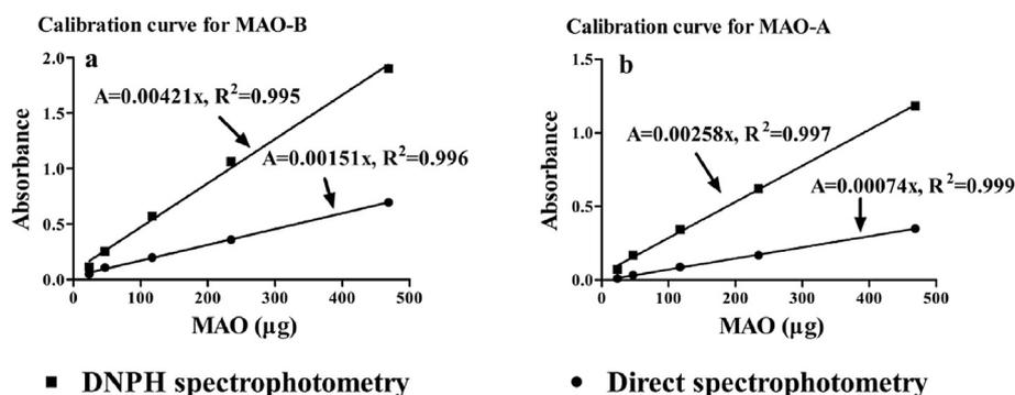
**Fig. 5.** Comparison of calibration curves for DNPH spectrophotometry (square) and direct spectrophotometry (circle). From left to right, the loads were 23.4, 46.9, 117, 234, 469  $\mu\text{g}$  of MAO protein. The graph shows that the regression equation for MAO-B and MAO-A are  $A = 0.00421x$ ,  $R^2 = 0.995$  and  $A = 0.00258x$ ,  $R^2 = 0.997$  by DNPH spectrophotometry and  $A = 0.00151x$ ,  $R^2 = 0.996$  and  $A = 0.00074x$ ,  $R^2 = 0.999$  by direct spectrophotometry.
