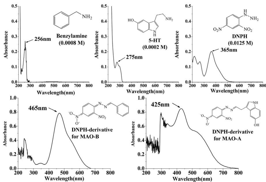
**Fig. 2.** Absorption spectra (800 nm–200 nm) of 5-HT (0.0002 M), benzylamine (0.0008 M), DNP (0.0125 M), DNPH-derivatives for MAO-B and MAO-A, and the MAO protein were 234.3 and 468.5  $\mu\text{g}$ , respectively, to obtain DNPH-derivatives for MAO-B and MAO-A. The graph shows that the absorption peaks are at 275 nm, 256 nm, 365 nm, 465 nm and 425 nm, respectively.
