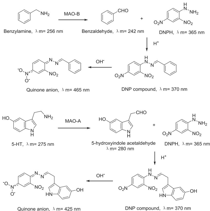
**Fig. 1.** The reaction scheme for catalytic oxidative deamination of monoamines and DNP derivatives of target aldehydes (benzaldehyde or 5-hydroxyindole acetaldehyde).
