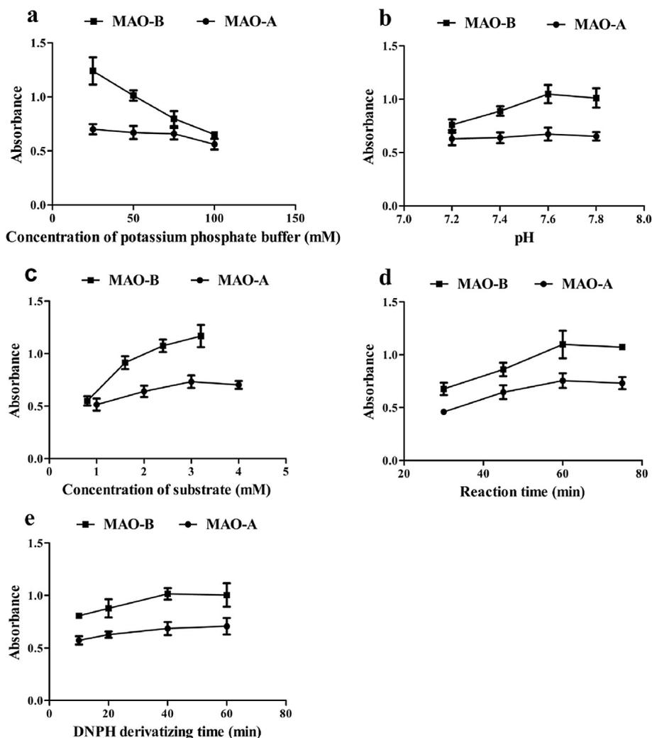
**Fig. 3.** Effects of reaction conditions of DNP spectrophotometry on MAO activity. a, concentration of potassium phosphate buffer; b, pH of potassium phosphate buffer; c, concentration of substrate (benzylamine or 5-HT); d, reaction time and e DNP derivatizing time. The absorbance are the mean of four samples and the results are shown as mean  $\pm$  SD (n = 4).
