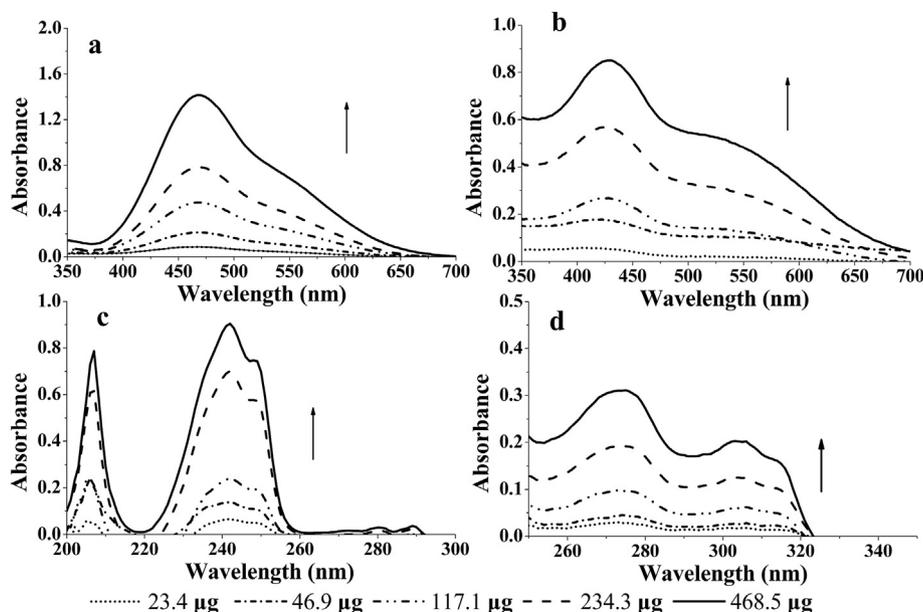
**Fig. 4.** The increasing concentration of MAO protein results in a corresponding increasing in absorbance by DNPH spectrophotometric method (a,b) and direct spectrophotometric method (c,d).
