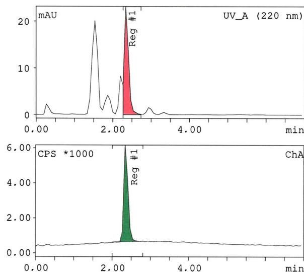
**Figure 5.** A typical chromatogram (method C) of crude product  $[^{18}\text{F}]$ FECNT ( $[^{18}\text{F}]$ -**8**) co-injected with non-radioactive standard. Top, UV (220 nm) detection; bottom, radioactivity detection. This figure is available in color online at [wileyonlinelibrary.com/journal/jlcr](http://wileyonlinelibrary.com/journal/jlcr)
