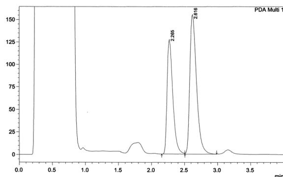
**Figure 1.** HPLC typical analytical chromatogram (method C) of the *N*-mesyloxy- derivative **10** reaction with fluoride (3 h, 80°C). Peak A, FECNT (**8**, Rt 2.26 min); peak B, side-product (Rt 2.62 min).
