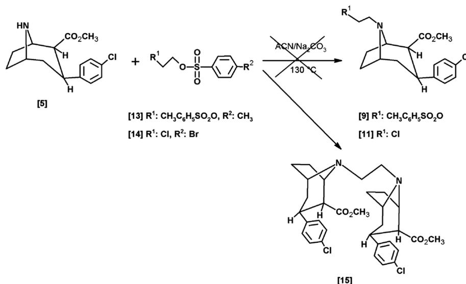
**Scheme 4.** Synthesis of 1,2-di-[2 $\beta$ -carbomethoxy-3 $\beta$ -(4-chlorophenyl)]nortropanyl]ethane (**15**).
