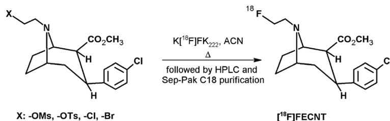
**Scheme 1.** One-step radiosynthesis of [<sup>18</sup>F]FECNT.
