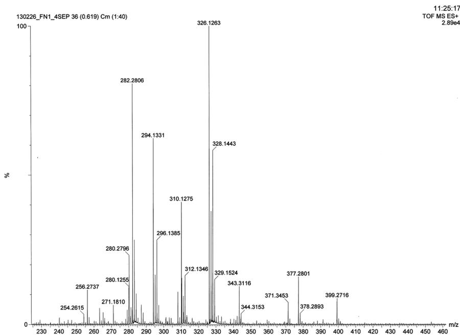
**Figure 2.** Mass spectrum of the compound corresponding to peak A (Rt 2.26 min, Figure 1), confirming the identity of FECNT.
