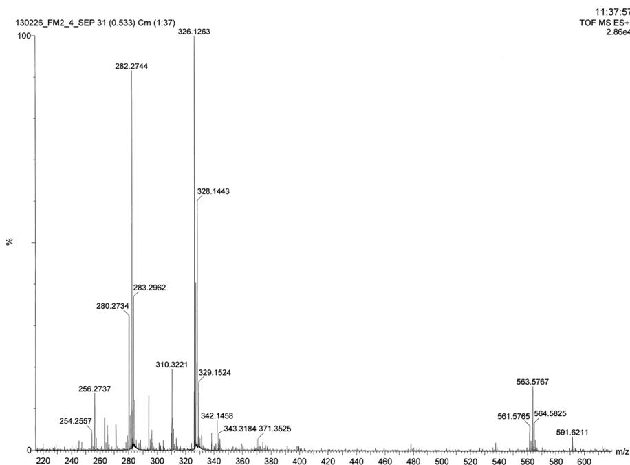
**Figure 3.** Mass spectrum of the compound corresponding to peak B (Rt 2.62 min, Figure 1), a side-product of the reaction with the same mass as FECNT.
