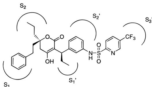
**Figure 6.** PNU-140690 illustrating the five enzymatic pockets binding mode.
