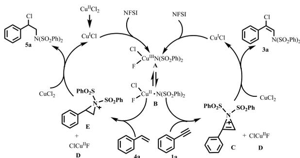
**Scheme 3.** The possible aminochlorination reaction mechanism of alkynes and alkenes.
