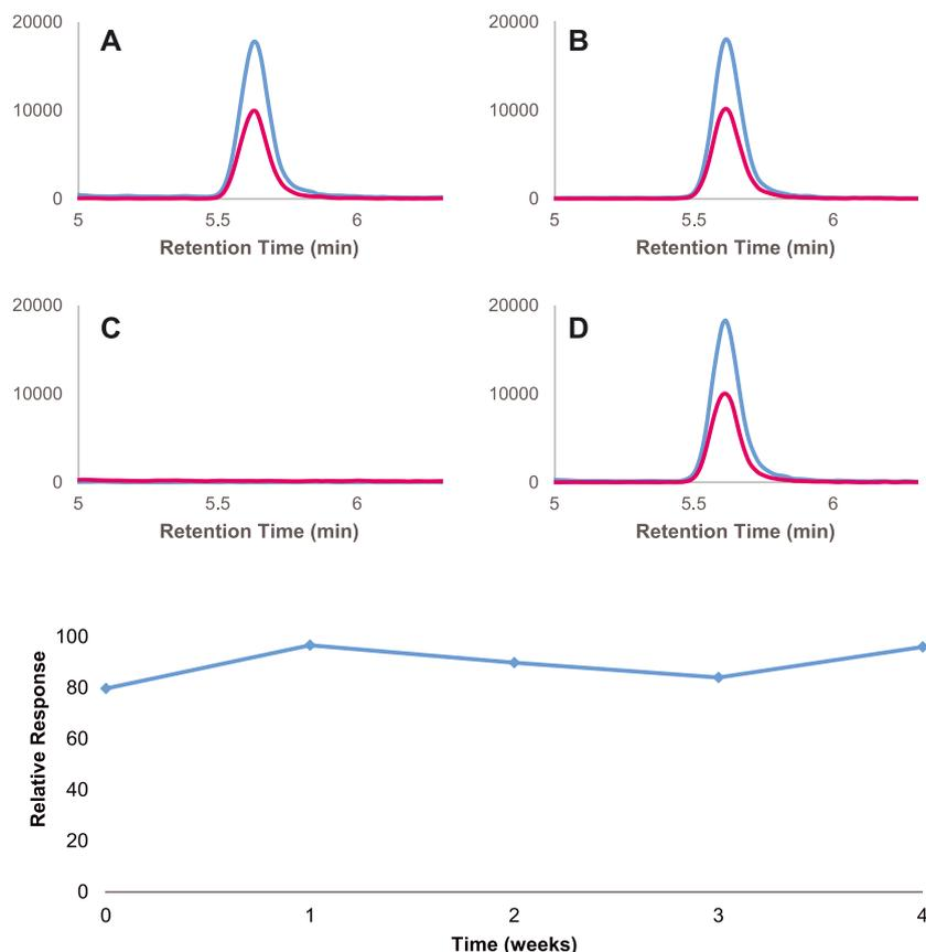
**Figure 2.** Nitenpyram is stable in surface (A) and ground waters (B). Degradation of nitenpyram in unpreserved finished drinking water (C). The nitenpyram response remains after fortification in finished drinking water with the addition of a  $NaS_2O_3$  (D). Chromatograms are shown with quantifier (blue) and qualifier (pink) MRM transitions overlaid. Nitenpyram is stable for 4 weeks in  $NaS_2O_3$ -preserved finished drinking water (bottom).
