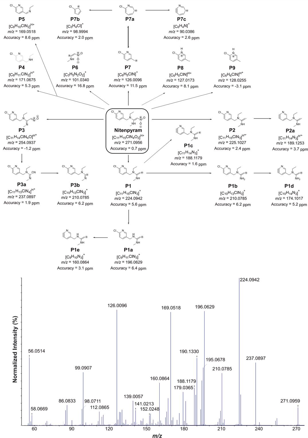
**Figure 3.** Nitenpyram fragmentation analysis (top) and the nitenpyram product ion spectrum (bottom) that was acquired with a collision energy (CE) of  $35 \pm 15$  V. Proposed primary fragments are denoted P1 → P9. Higher order fragments are denoted by a lower case letter (e.g., P3a).
