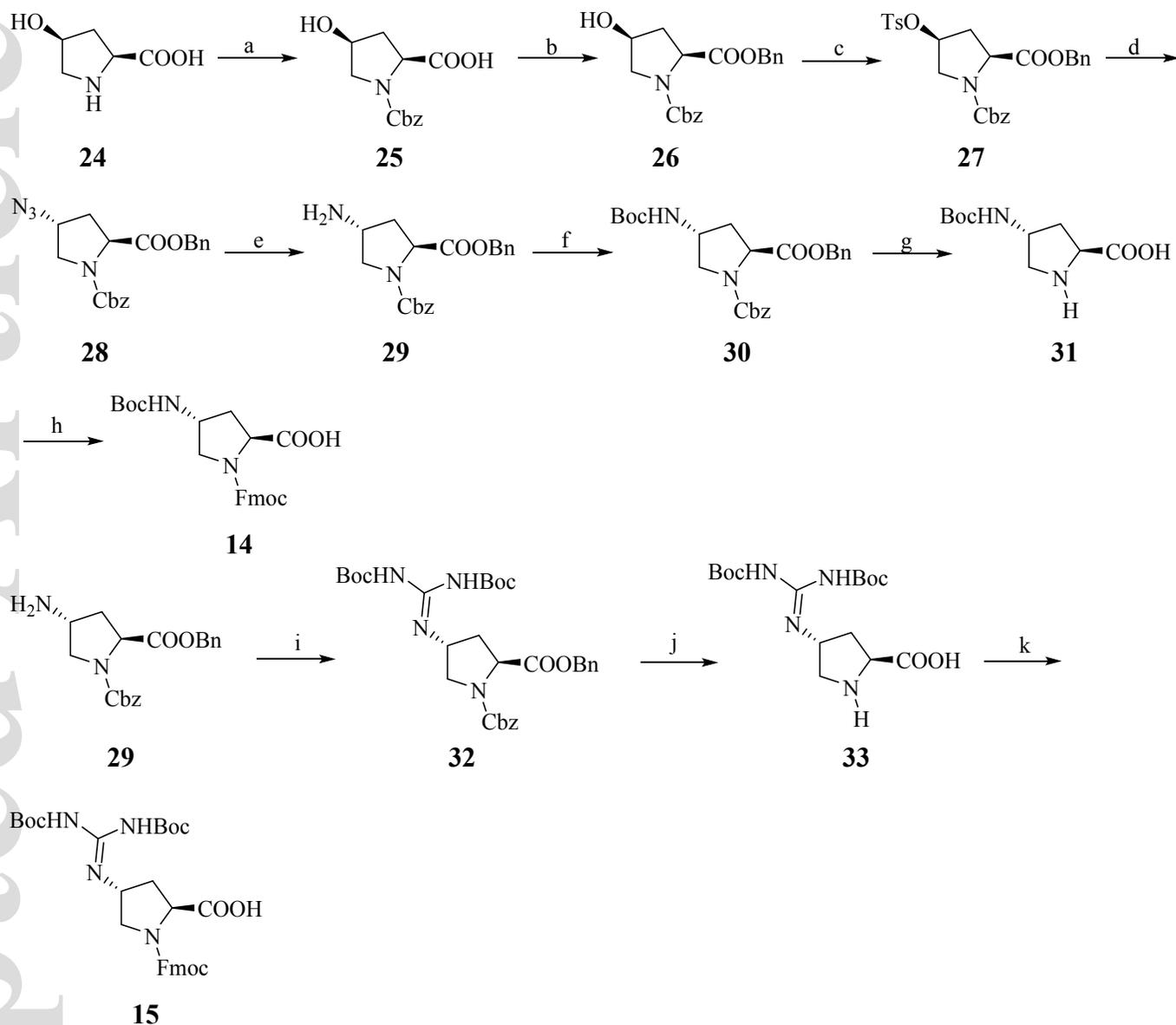
Scheme 2. Synthesis of *trans*-4-BocNH- $N^a$ -Fmoc-Pro-OH (**14**) and *trans*-4-(diBoc-gunidino)- $N^a$ -Fmoc-Pro-OH (**15**).
