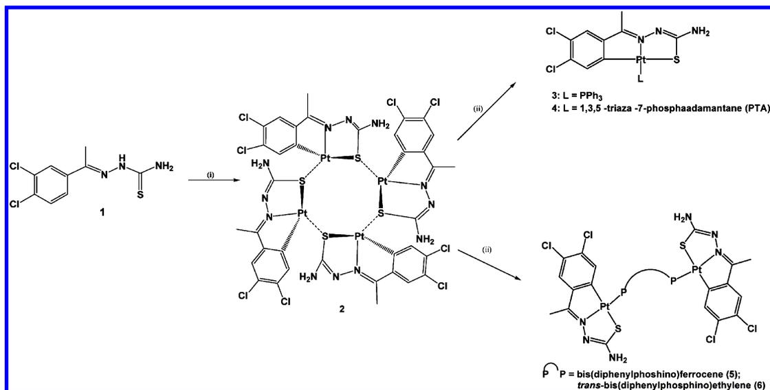
Reaction conditions: (i) K<sub>2</sub>[PtCl<sub>4</sub>], EtOH–H<sub>2</sub>O, 50 °C, 5 days; (ii) L or P<sup>^</sup>P, acetone, room temperature, 3 h.
