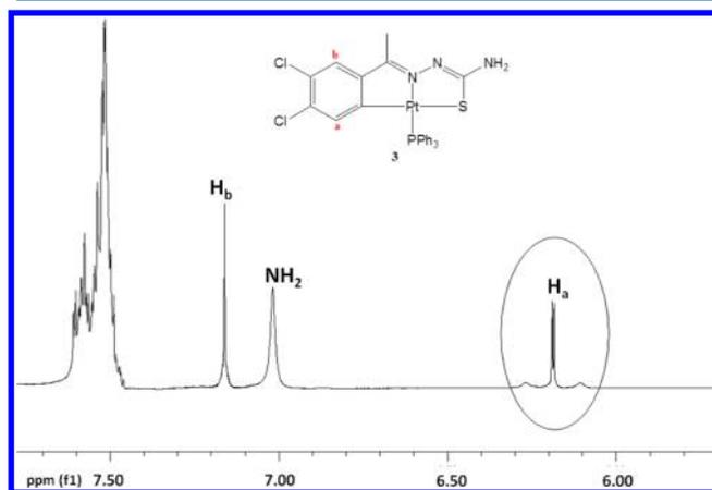
**Figure 1.** Expansion of the <sup>1</sup>H NMR aromatic region of complex 3. The proton resonance with Pt satellites is circled.
