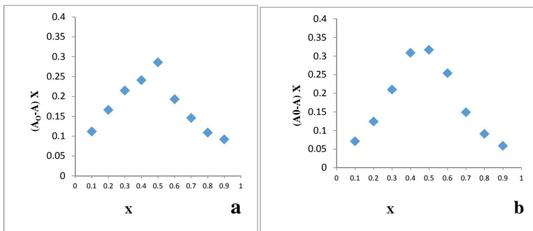
**Figure 4.** Job's plot of monomeric heme complex formation with compound **7o**; **a**) at pH 5.6; **b**) at pH 7.4;  $X$  (mole fraction of compound **7o**) =  $[\text{Compd. } \mathbf{7o}]/([\text{Compd. } \mathbf{7o}] + [\text{heme}])$ ;  $A_0$  is the absorbance, when  $x = 1$  and  $A$  is the absorbance at respective values of  $x$
