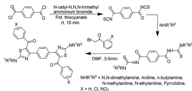
Scheme 6 General synthesis of 4,4'-(1,4-phenylene)bis(1,3-thiazole) derivatives (6a–6f).
