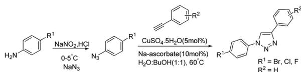
Scheme 3 General synthesis of 1,4-disubstituted-1,2,3-triazole derivatives (5a–5c).
