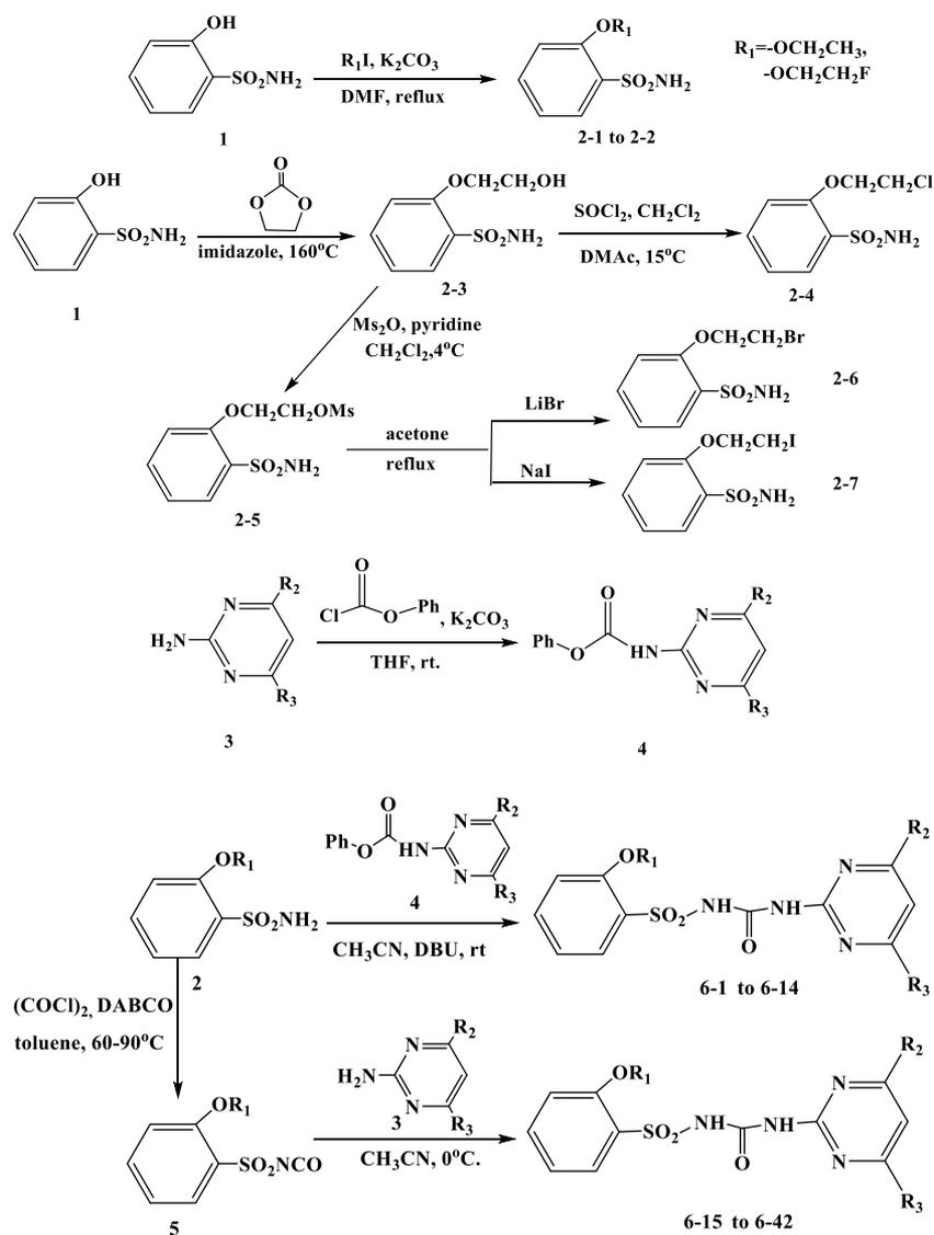
**Figure 3.** Synthetic routes of the intermediates and the target sulfonylurea compounds.
