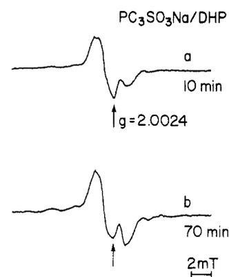
**Figure 3.** ESR spectra at 77 K from  $PC_3SO_3Na$  in DHP vesicles after photoirradiation for 10 and 70 min. Arrows indicate the peaks due to  $AP^+$ .
