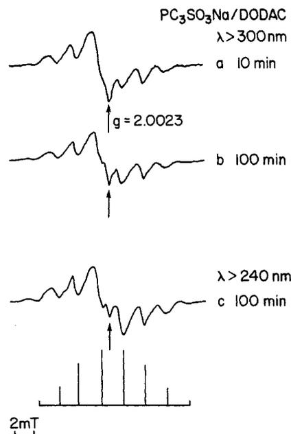
**Figure 5.** ESR spectra at 77 K from PC<sub>3</sub>SO<sub>3</sub>Na in DODAC vesicles after photoirradiation for (a) 10 min, (b) 100 min with a WG320 filter, and (c) 100 min with a Corning 7-54 filter. The stick diagram shows an idealized octet spectrum of the surfactant radical. Arrows indicate AP<sup>+</sup> radicals.
