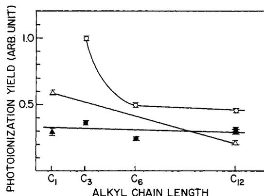
**Figure 6.** Photoirradiation yield at 77 K from alkylphenothiazines in vesicles for 10 min of irradiation with a WG320 filter versus the alkyl chain length. The symbols (○) and (△) show PC<sub>n</sub>SO<sub>3</sub>Na ( $n = 3, 6, 12$ ) and C<sub>m</sub>PSO<sub>3</sub>Na ( $m = 1, 12$ ) in DODAC vesicles while (●) and (▲) show PC<sub>n</sub>SO<sub>3</sub>Na and C<sub>m</sub>PSO<sub>3</sub>Na in DHP vesicles. The error bars indicate the average deviation of three or more measurements.
