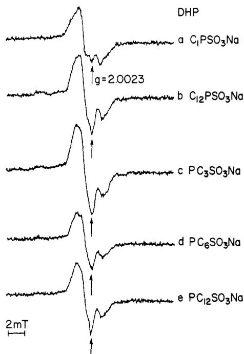
**Figure 1.** ESR spectrum at 77 K from various alkylphenothiazines in DHP vesicles after 10 min of photoirradiation with a WG320 filter ( $\lambda > 300$  nm). The arrows indicate  $AP^+$  radicals.
