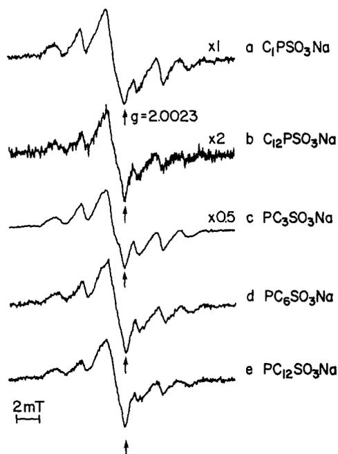
**Figure 4.** ESR spectra at 77 K from various alkylphenothiazines in DODAC vesicles after 10 min of photoirradiation with a WG320 filter. The arrows indicate AP<sup>+</sup> radicals.
