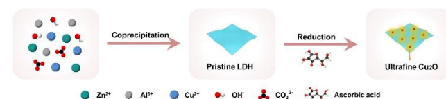
Scheme 1. Synthetic strategy used to prepare LDH-supported sub-3 nm ultrafine \text{Cu}_2\text{O} .
