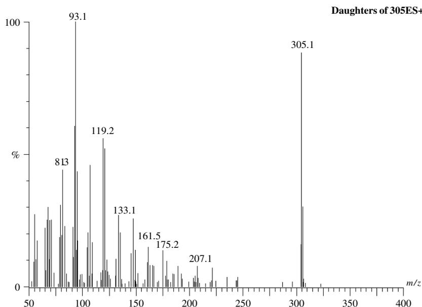
**Figure 3.** ESI product ion spectrum of  $[M+H]^+$  at  $m/z$  305 for AA (CE=30 eV).
