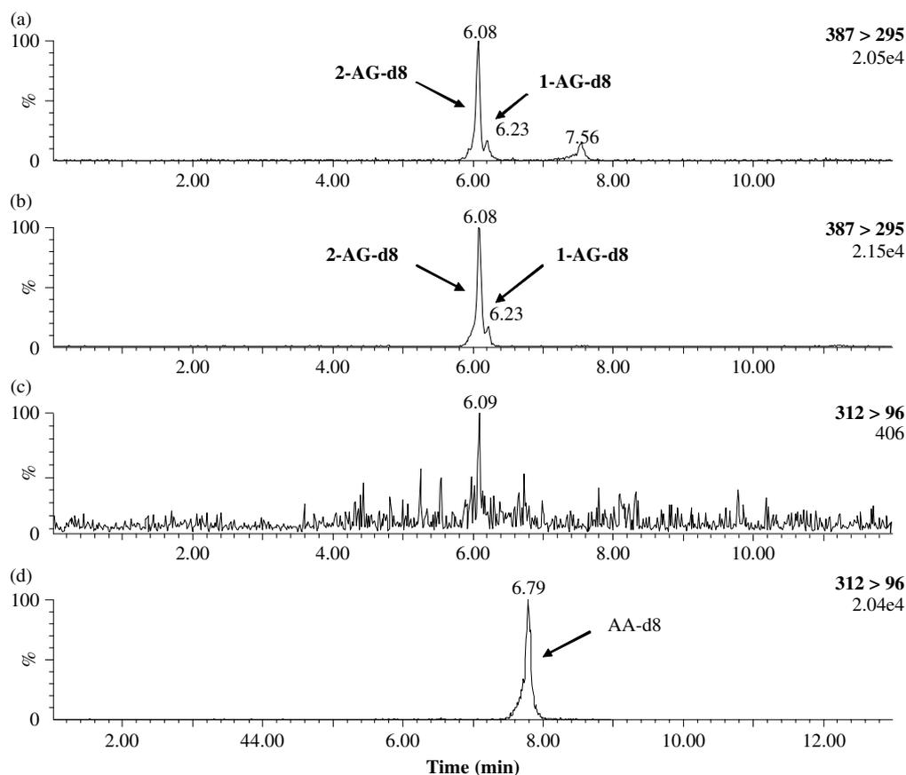
**Figure 1.** The MRM ion chromatograms of: a) 2-AG-d8 and 1-AG-d8 from the mouse brain tissue extracts spiked with 2-AG-d8, b) 2-AG-d8 and 1-AG-d8 from the ACN solution of 2-AG-d8, c) AA-d8 from the mouse brain tissue extracts spiked with 2-AG-d8 and d) AA-d8 from the ACN solution of AA-d8.
