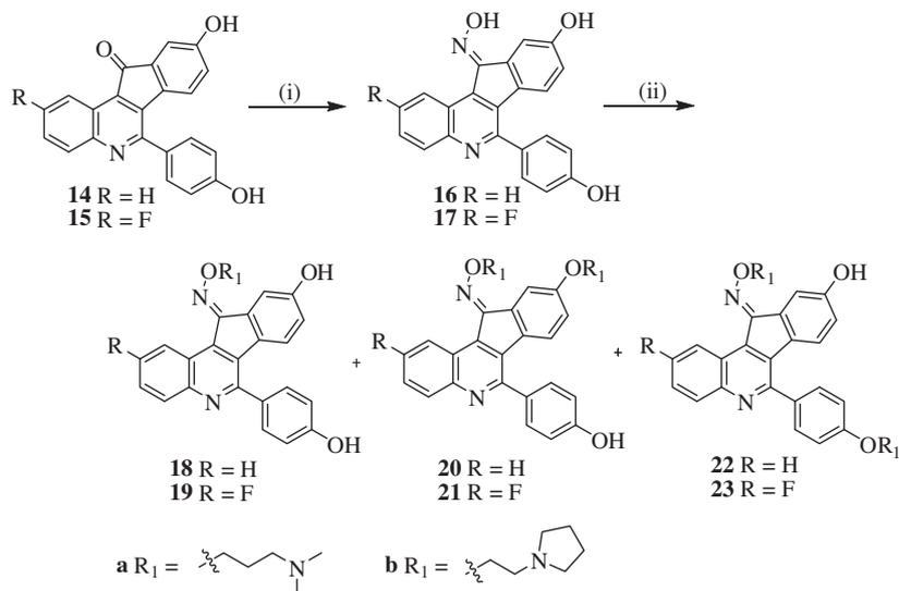
**Scheme 2.** Reagents and conditions: (i) Hydroxyamine, 2-EtOH, 150 °C, 3 h; (ii) NaH, alkyl halides, DMF, 80 °C, 25 min.
