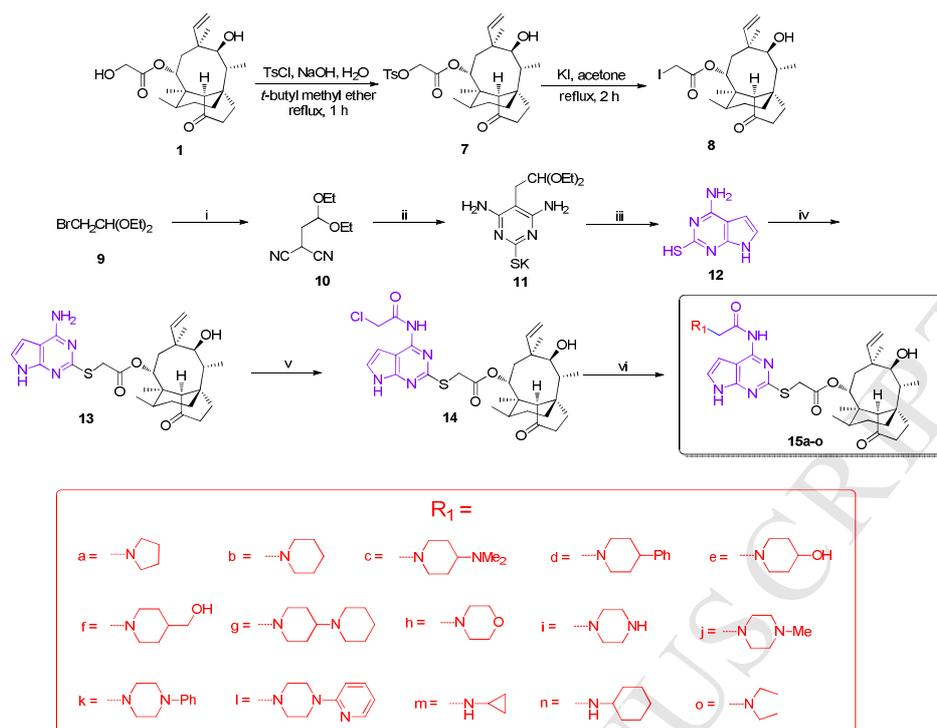
**Scheme 1.** Reagents and conditions: (i) malononitrile,  $K_2CO_3$ , DMF, 50 °C, overnight; (ii) thiourea, *t*-BuOK, EtOH, 80 °C, overnight; (iii) 4 N HCl for 1 h and 4 M NaOH for 10 min; (iv) compound **8**, 15% NaOH, THF, 0 °C, 2 h; (v) chloroacetyl chloride,  $Et_3N$ , DCM/DMF = 5/1, rt, 2 h; (vi)  $R_1H$ , 2 mol% NaI,  $K_2CO_3$ , THF, 60 °C.
