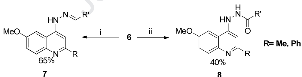
Scheme 2. Synthetic pathways for 4-hydrazonequinoline 7 and 4-hydrazidequinoline 8 derivatives: Reagents: (i) R'C(O)H, (ii) R'COCl.
