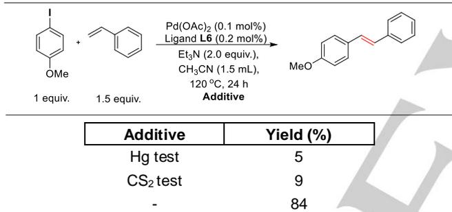
**Scheme 7:** Catalyst poisoning study for the presence of heterogeneous or nanoparticular pathway.
