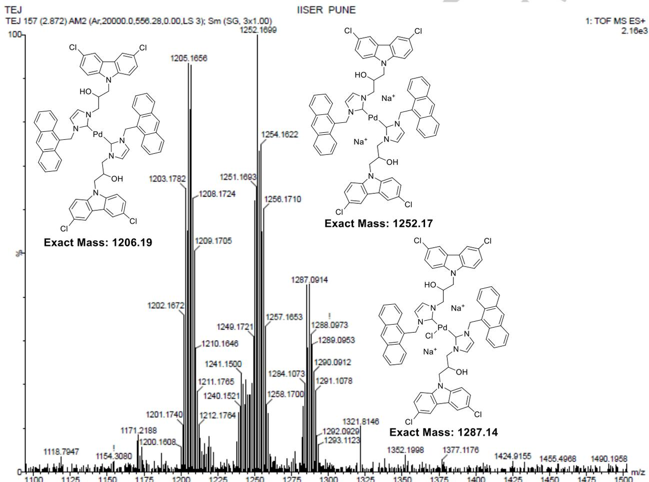
**Figure 3:** HRMS analysis of reaction mixture for the detection of Pd species in solution.
