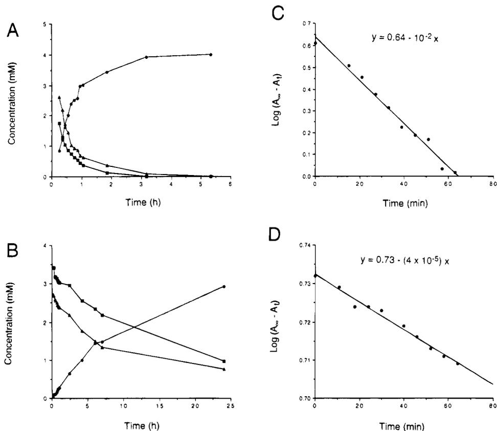
**Figure 6.** Representative plots of the time dependence (A, B) and pseudo-first-order kinetics (C, D) of OX formation from BEA and CEA (each 5 mM) in the presence of a 20-fold initial excess of  $\text{HCO}_3^-$ . Experimental procedures are described in Materials and Methods. Key to plots: (A) ■ BEA, ▲ BEA carbamate, ● OX; (B) ■ CEA, ▲ CEA carbamate, ● OX.
