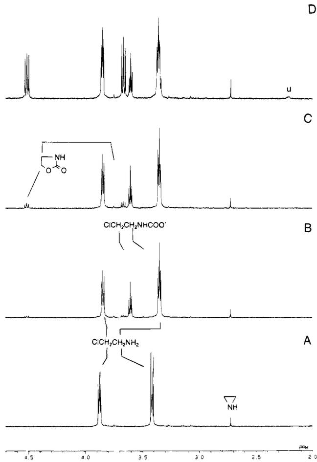
**Figure 3.** Partial 500 MHz  $^1\text{H}$  NMR spectra ( $\delta$  2.0–4.7) of a standard solution of CEA in  $^2\text{H}_2\text{O}$  (A) and a model solution of CEA in the presence of 20-fold excess of  $\text{HCO}_3^-$  in  $^2\text{H}_2\text{O}$ . Spectra illustrated were acquired 30 min (B), 1 h (C), and 7 h (D) following reaction initiation. Note pH shift of position of CEA on changing to  $\text{HCO}_3^-$  solution. Experimental procedures are described in Materials and Methods.
