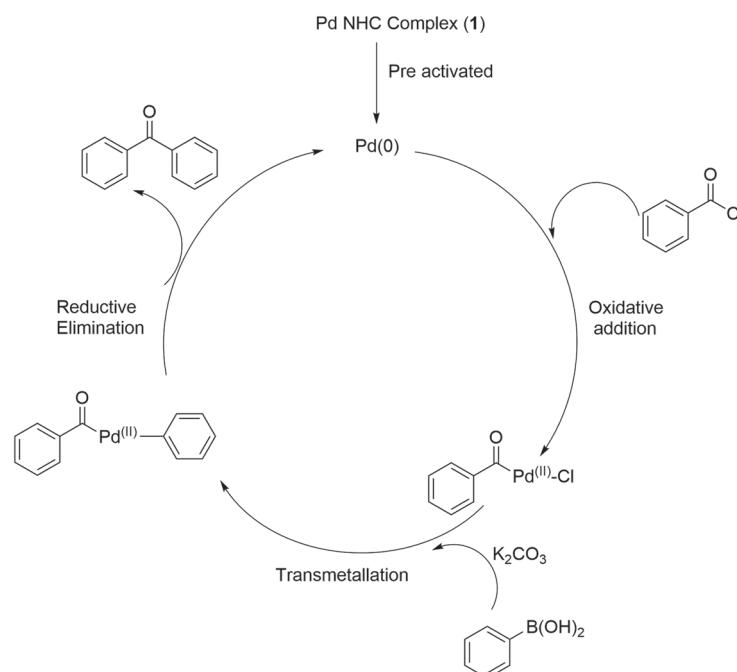
**S C H E M E 3** Probable mechanism for acylative cross-coupling reaction. NHC, N-heterocyclic carbene
